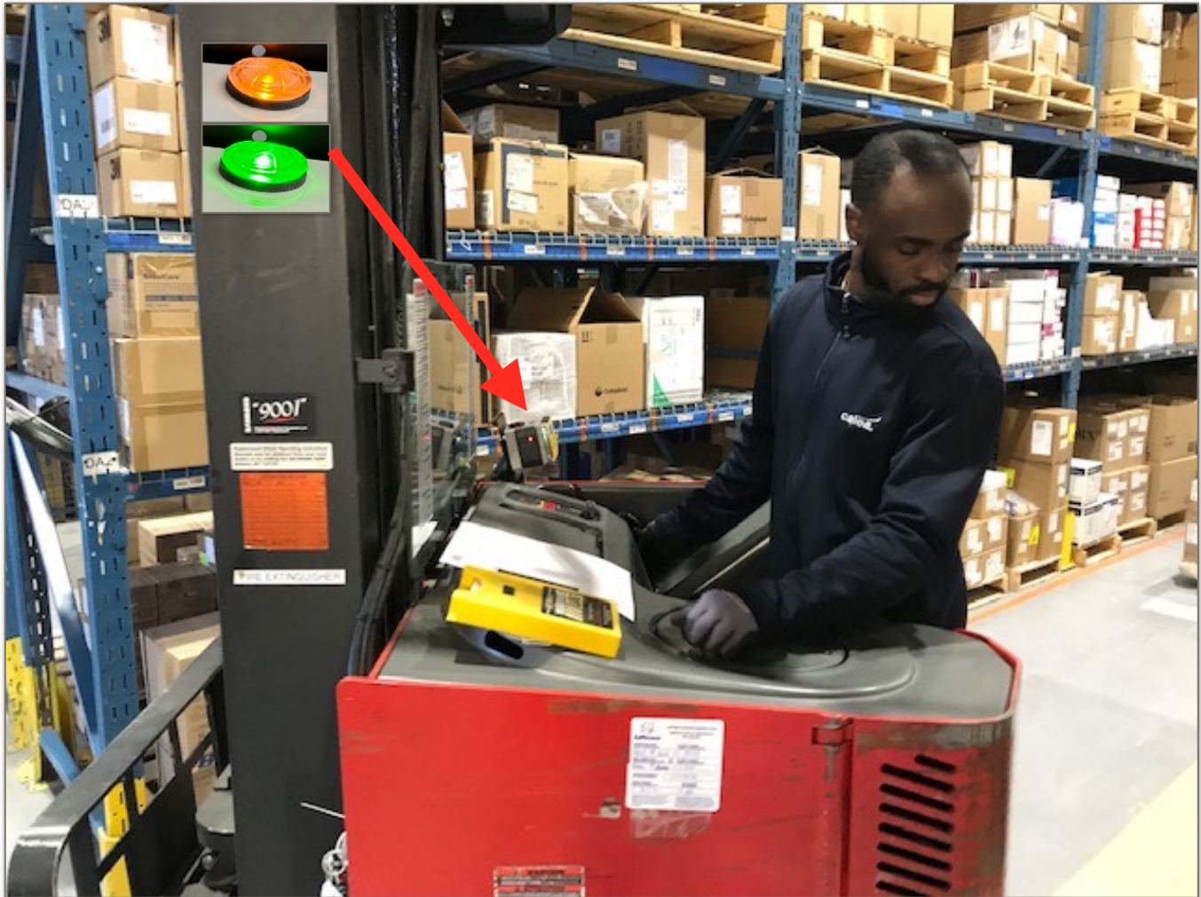
Stand Alone Decentralized Lift Truck Operator Access Control With Fully Automatic Daily OSHA / Pre-shift Safety Check Recorder
