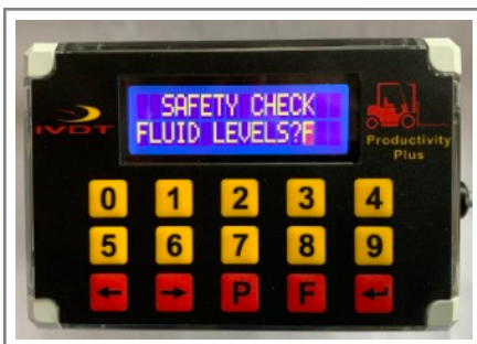
Stand Alone Decentralized Lift Truck Operator Access Control With Fully Automatic Daily OSHA / Pre-shift Safety Check Recorder
