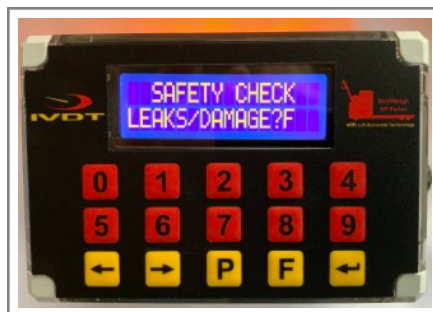
Stand Alone Decentralized Lift Truck Operator Access Control With Fully Automatic Daily OSHA / Pre-shift Safety Check Recorder
