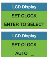
Use left ◀ and right ▶ arrow key (bottom left side of the keypad) to change from AUTO to MANUAL date/ time set up.
