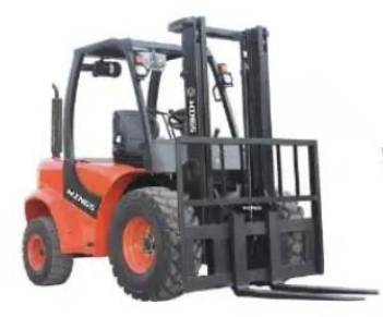
Rough Terrain Forklift
